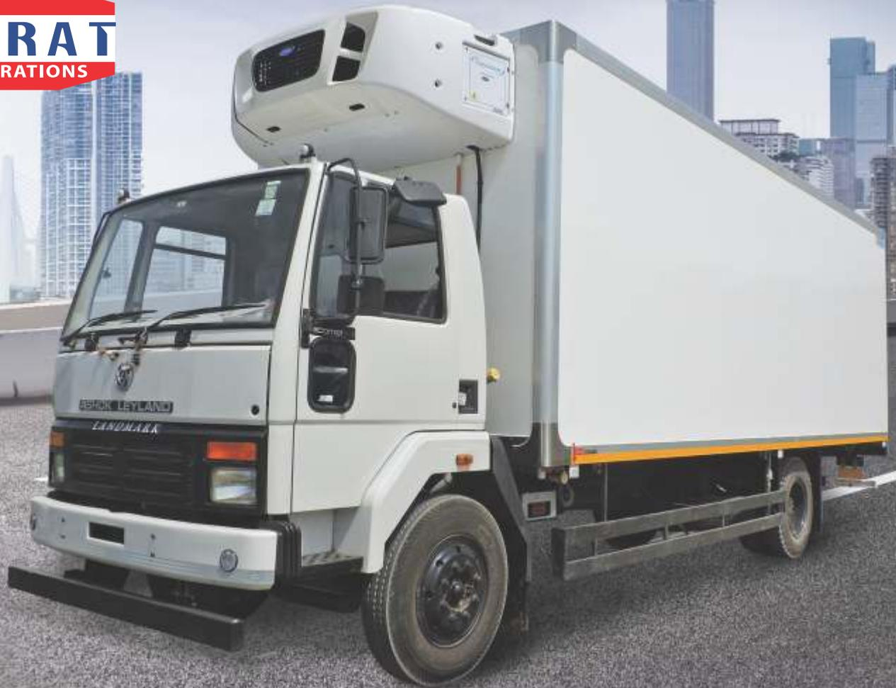
Bharat Refrigerations Refrigerated container is designed to transport with options of different temperature range (+15°C to -25°C) for all perishable foods on all type of vehicle such as small, mini truck & heavy loading truck.
